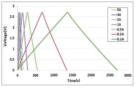
Charge-Discharge Rate Test
